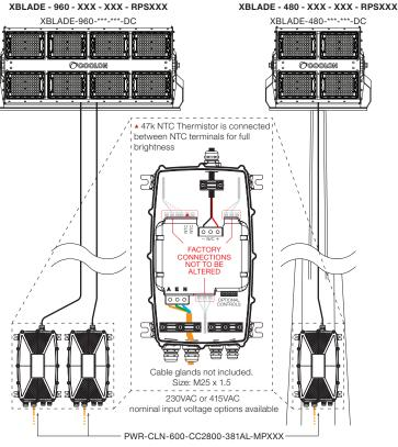
Distance between the power supply and luminaire can be extended up to 100 metres using 1.5mm<sup>2</sup> cable.
